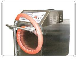
The 75 gallon unit stores about <u>eleven</u> 50lb fryer's worth of oil! The GreaseVAC can extract the oil while it is hot. No time wasted waiting for the oil to cool.
