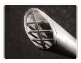
The nozzle has a safety screen to keep large objects from clogging hose.
